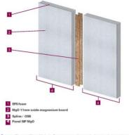
Fasteners are applied through MgO board into the spines, top and base plate
